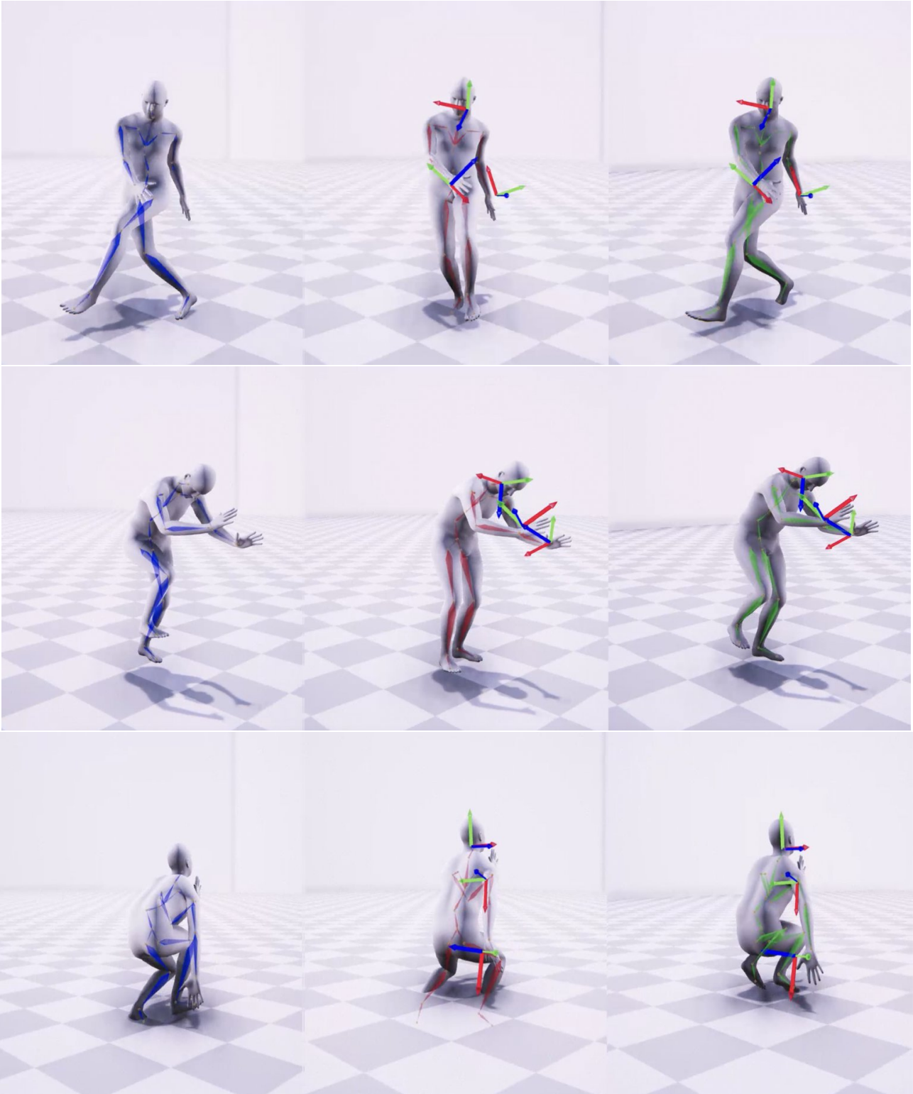
Figure 1. Qualitative comparison on test sequences from AMASS dataset. We visualize the predicted skeletons and human body meshes: (a) Ground truth skeletons in blue, (b) AvatarPoser predictions in red, (c) AGRoL predictions in green. It can be seen that our predicted motion is more accurate compared to the predictions of AvatarPoser, especially in the lower body. RGB axes illustrate the location and orientation of the head and hands provided as input to the models. Please refer to our project page for more qualitative results.
