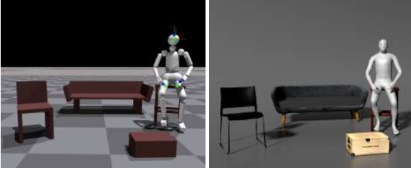
Fig. 3. For accurate contact behavior we approximate all the real shapes (right) with geometric primitives (left): The character’s mesh is approximated with 18 collision geometries (capsules, boxes and spheres). The environment objects are similarly approximated with geometric primitives. As long as the contact surfaces match, the visualization will look accurate. We calculate masses and inertias of the character and objects based on their collision geometry and assuming uniform density.
