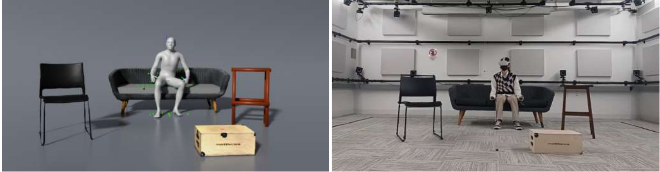
Fig. 1. From only the pose of a headset and controllers, our method reconstructs a matching full-body pose that interacts naturally with various objects in a simulated environment.
