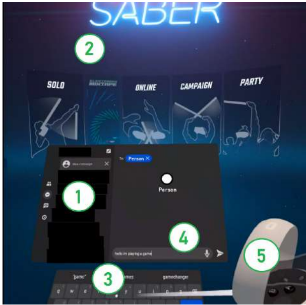
Figure 2: Attack scenario. (1) The foreground app (Facebook Messenger) displays on top of the (2) background app (Beat Saber), which continues to render using real-time head motion tracking. (3) The victim types messages using the system keyboard into the (4) text entry field. (5) The controller inputs are not available to background app (2) while the foreground app is open.
