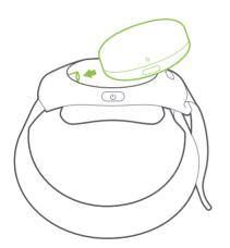
① Once the tracker is connected to the USB-C socket of the base, press and fix it in the base.
