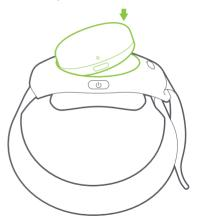
② Press the Eject button for the tracker to detach.
