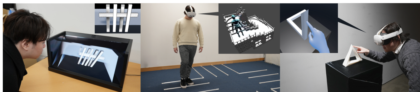
Figure 1: (Left) Observing an impossible object of the wrong depth using a stereoscopic display. (Center) A user ascending the stairs is seen from the outside. The tactile feedback on their feet enhances the illusion of continuous ascending. (Right) The user can interact with an impossible object in VR by touching the corresponding planes in physical space.
