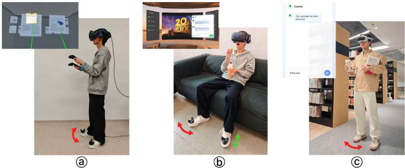
Figure 10: Potential application scenarios of AnkleType. (a) A user is browsing and managing content in a VR workspace. He grasps and holds two documents using controllers with his left and right hands by pulling the triggers. He can input the virtual sticky notes via AnkleType without putting the document down. (b) A user is sitting and watching a VR movie with one hand holding a bag of potato chips while the other hand is engaged in eating. He can input text via AnkleType to respond to notifications without clearing his hands. (c) A user wearing an MR HMD is walking in a library with books and coffee in both hands. He can quickly respond to short messages using AnkleType without freeing his hand and leaving his eye off the surroundings.
