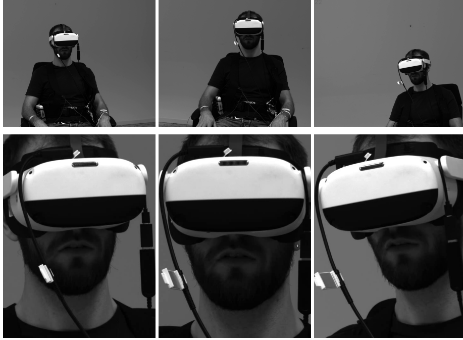
Figure 2: Example frames from each monochrome camera view (left, center, right): raw frames (top) and YOLO Pose lower-face crops (bottom) at the same timestamp.
